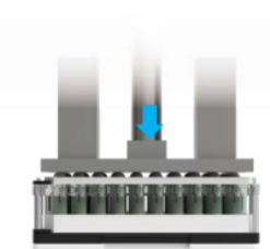
STEP 6 Press with machine to seal off the filled devices.
