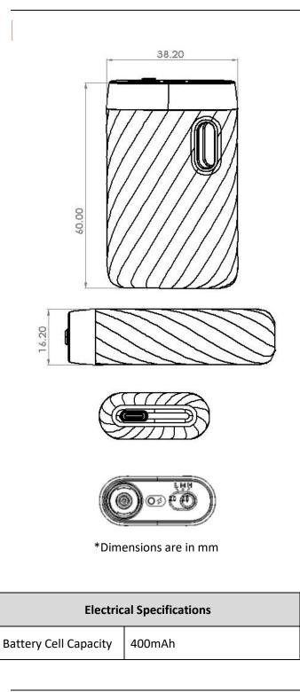
Output Voltage with<br/>1.4Ω loadSetting 1: 2.8Vrms<br/>Setting 2: 3.2Vrms<br/>Setting 3: 3.6VrmsMax. Current Output3AMax Charging<br/>Current500 mAActivation Time0 – 10 seconds (± 2s)
