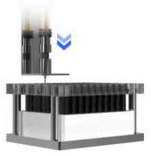
3. Place the pre-loaded mouthpiece tray on the deflector. Gently tramp down the mouthpieces to ensure they are aligned with the batteries.
