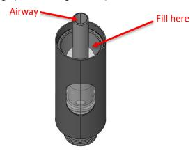
While the cartridge is oriented vertically with the threaded connector downward, fill the cartridge through the needle. Do not overfill.
