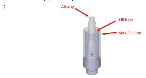
While the cartridge is oriented vertically with the threaded connector downward, fill the cartridge through the needle. Do not overfill.
